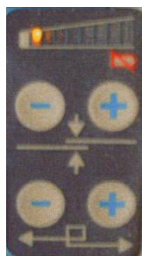
Li-Po storage battery almost empty
